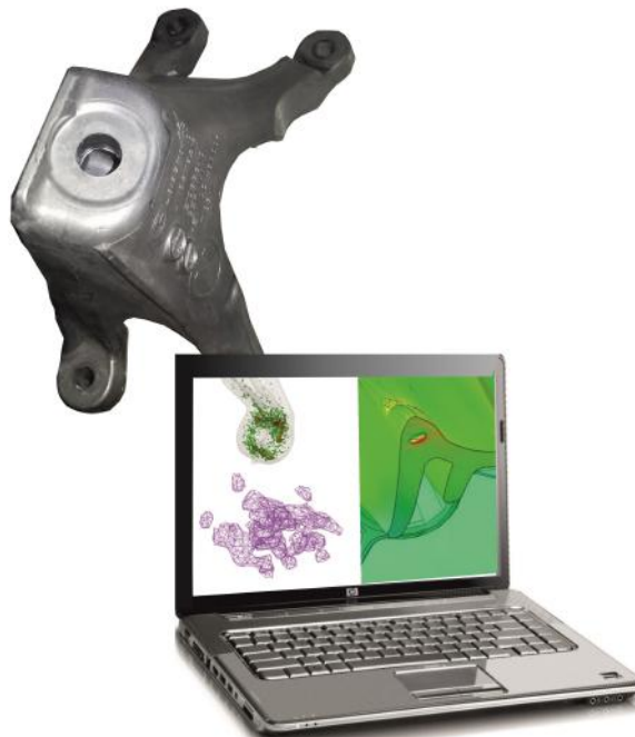
Figure 1: Cast part including micro-structural details in the simulation [2].
